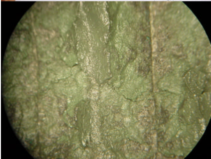
Figure 22: Deposits stuck in a failed radiator pressure cap.
