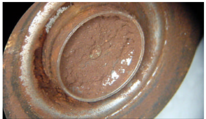
Figure 22: Deposits stuck in a failed radiator pressure cap.
